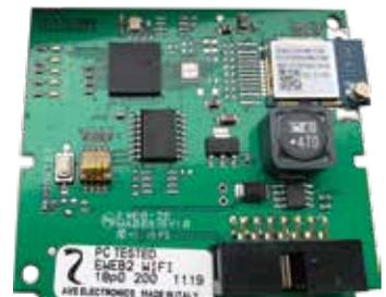
broadband network - Dynamic DNS management - LAN port: RJ45, 10/100 Mbit/s - Compatibility: CAPTURE, XTREAM control panels, XWIN and ELM software - IMQ-INCERT EN 50131 Grade 2 CERTIFICATION
