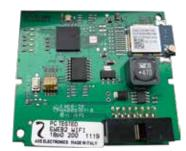
broadband network - Dynamic DNS management - LAN port: RJ45, 10/100 Mbit/s - Compatibility: CAP-TURE, XTREAM control panels, XWIN and ELM software - IMQ-INCERT EN 50131 Grade 2 CERTIFICATION
